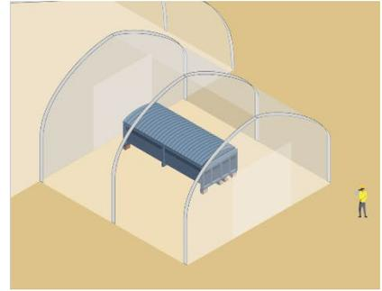
Fully sealed bins with Pit F waste will be pulled from the entry chamber and loaded onto haul trucks and transported to a permitted landfill the same day
