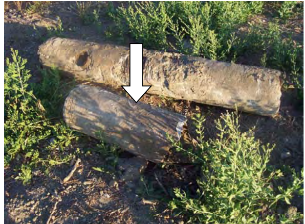
2. ACM 18" diameter Transite ® pipe section, located northwest of "Lagoon 2", approximately 3.5 feet in length (Sample I.D. TRANSITE-01 containing 30% Chrysotile). [Note: Rear pipe is non-suspect steel reinforced concrete.]
