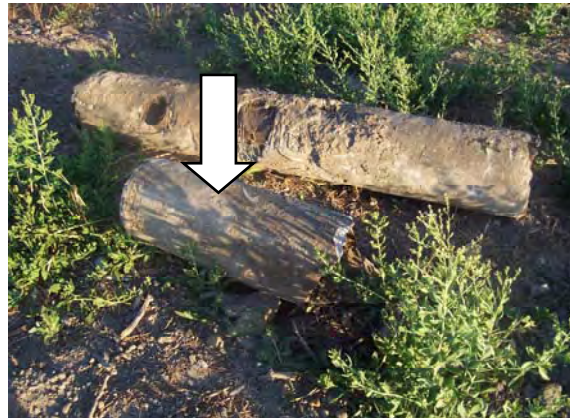
2. Subject Asbestos Cement Pipe. (Note: Object in rear is reinforced concrete.)
