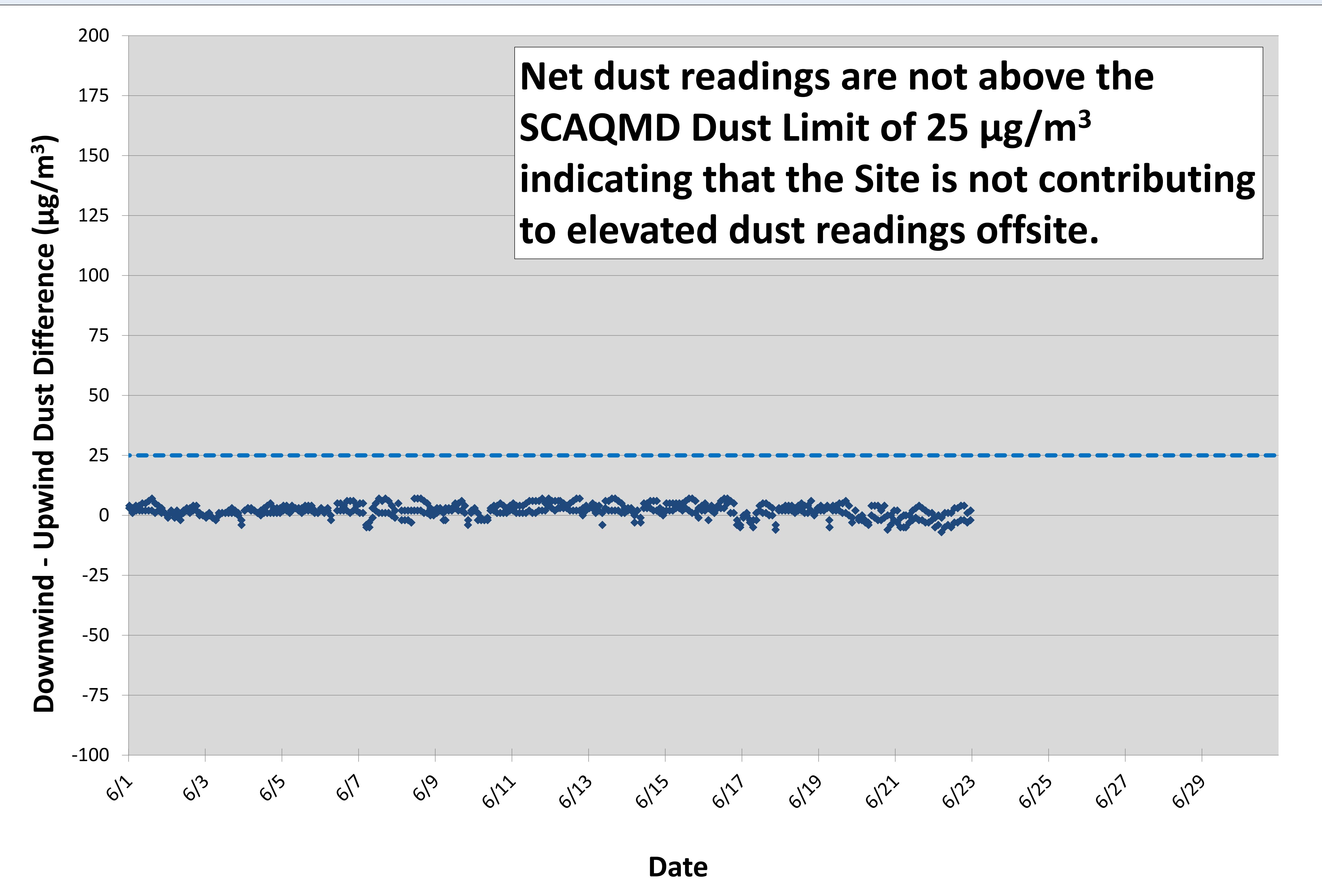
Net dust represents the dust that may be leaving the Site. This is determined by subtracting upwind data (dust blowing onto the Site from other sources) from downwind data. This helps us monitor that dust control actions are effective.
