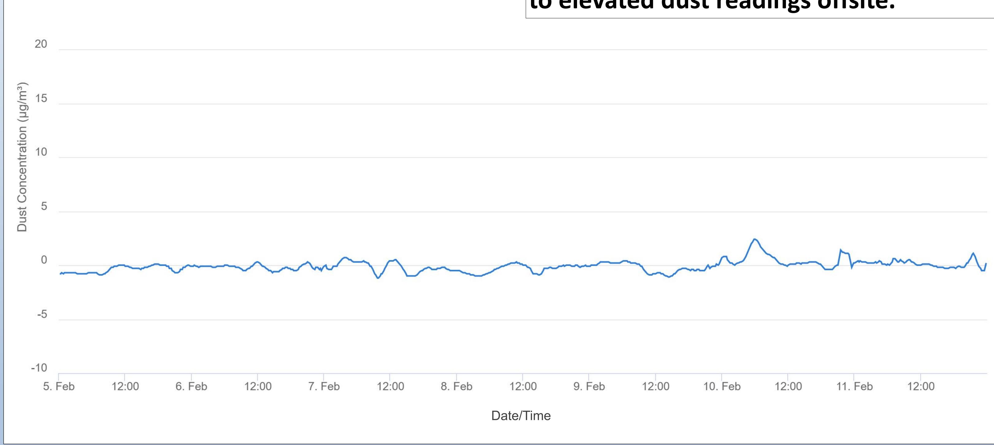
Net dust represents the dust that may be leaving the Site. This is determined by subtracting upwind data (dust blowing onto the Site from other sources) from downwind data. This helps us monitor that dust control actions are effective.
