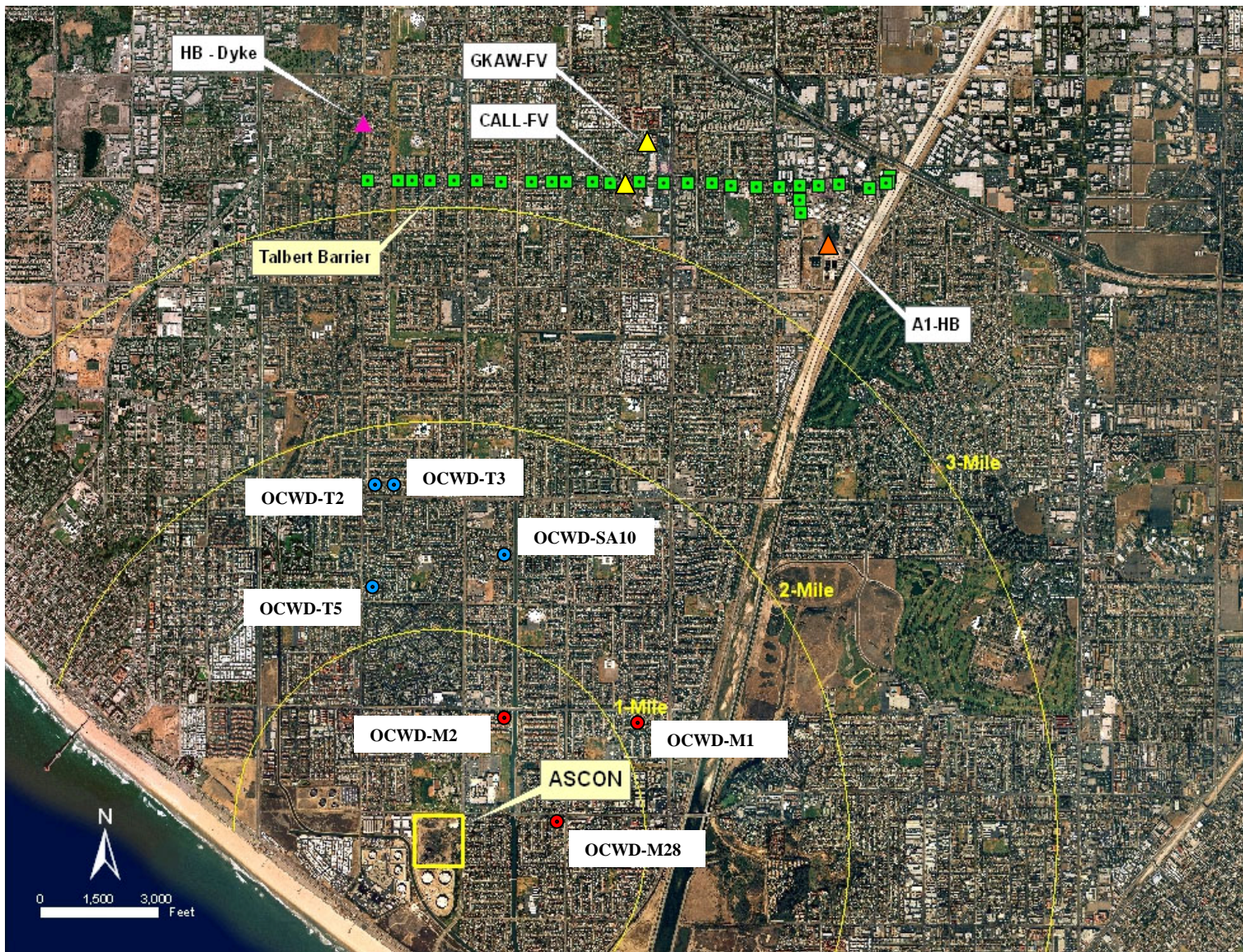
Distance to Drinking Water Wells and Selected Monitoring Wells in Talbert Gap Northwest of the Santa Ana River Figure 5-3 Source: Orange County Water District – Personal Communication Ascon Landfill Site, Huntington Beach, California March 2005
